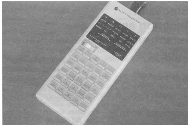
(b) A typical hand-held PLC programmer
